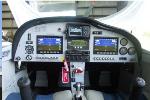
Cockpit with DYNON D100/D120 Upgrade
