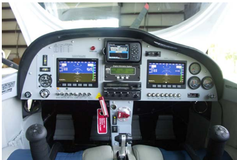
Figure 4. SportCruiser, with DYNON D100/D120 glass cockpit upgrade
